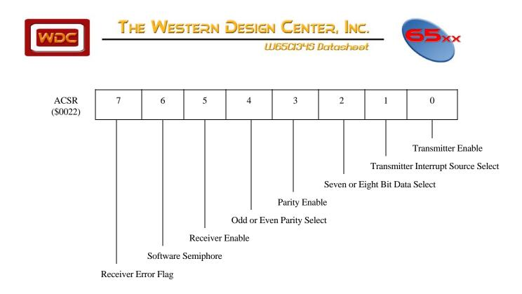
Figure 1-9 ACSR Bit Assignments
