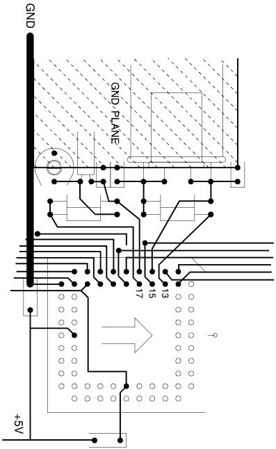
Figure 4-8 Circuit Board Layout for Oscillator Circuit
