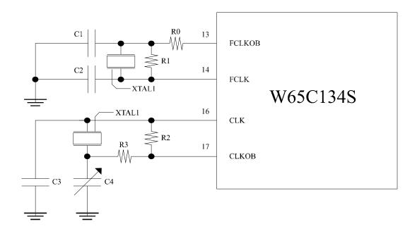
In constructing this oscillator circuit, components should be kept as physically close to the W65C134S as possible and any excess in component leads should be trimmed off.
