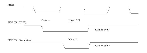
Figure 2-3 BE Timing Relative to PHI2
