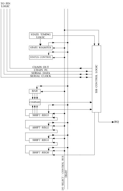
Figure 4-6 Serial Interface Bus (SIB) Block Diagram
