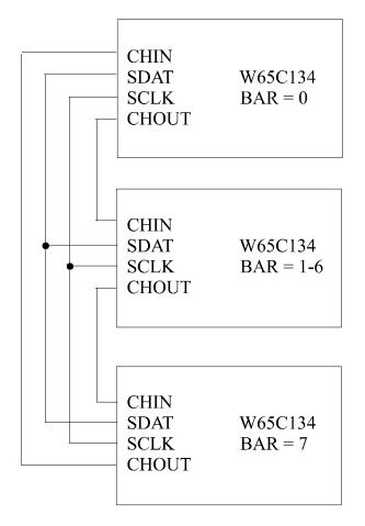
Figure 1-14 W65C134S Serial Interface Bus (SIB) Wiring Diagram
