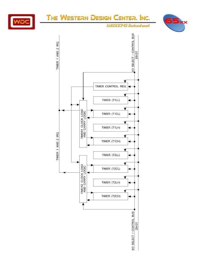
Figure 4-3 W65C134S timer 1 and 2 (T1 and T2) Block Diagram
