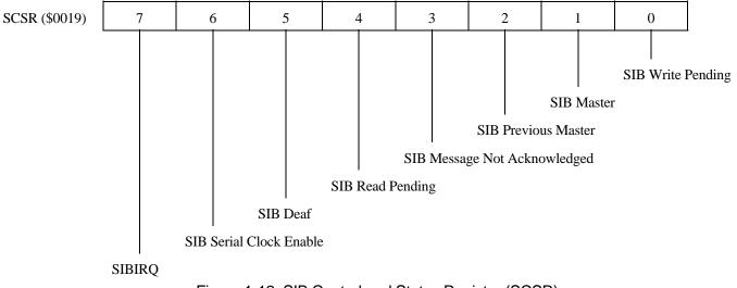
Figure 1-12 SIB Control and Status Register (SCSR)
