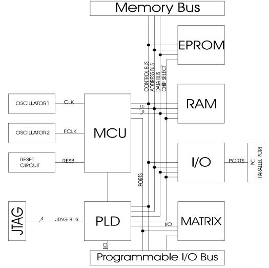
Figure 4-10 W65C134SPCB Embedded System Development Board Block Diagram
