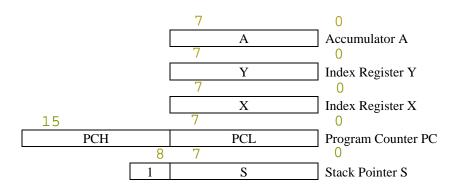
Figure 1-16 W65C02S Microprocessor Programming Model
