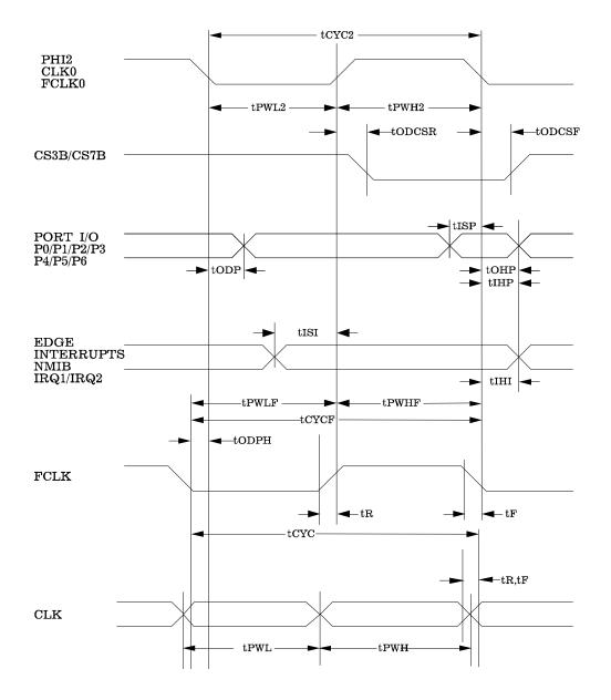
Figure 3-1 AC Timing Diagram #1
