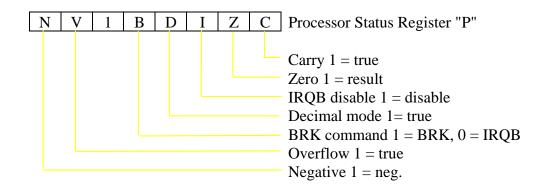
Figure 1-17 W65C02S Status Register Coding
