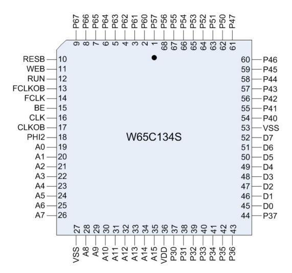
Figure 2-2 W65C134S 68 Lead Chip Carrier Pinout
