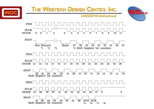
Figure 1-13 Serial Interface Bus (SIB) Message Transmission Timing Diagram
