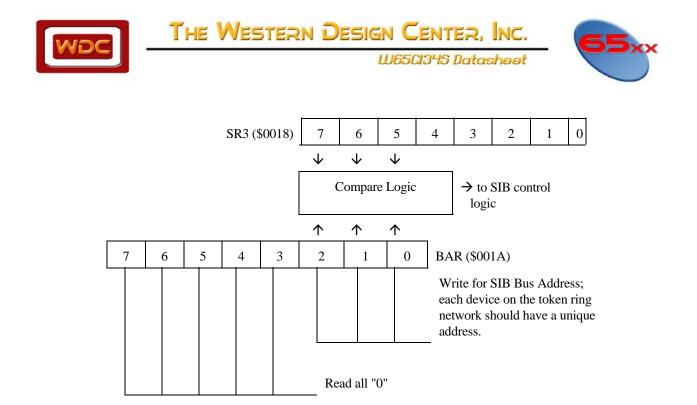
Figure 1-15 Bus Address Register (BAR)
