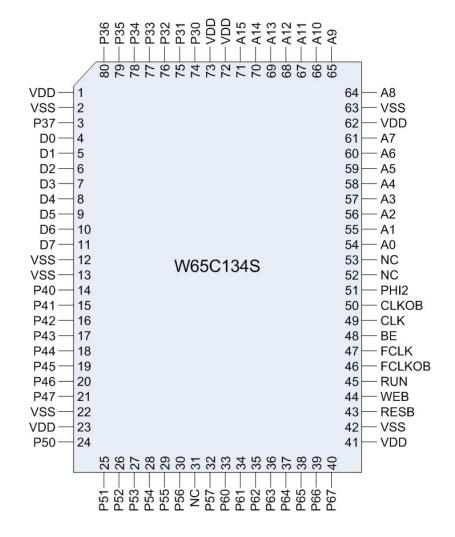
Figure 2-3 W65C134S 80 Lead Chip QFP Carrier Pinout
