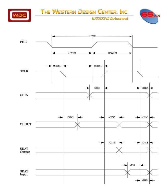
Figure 3-3 AC Timing Diagram #3
