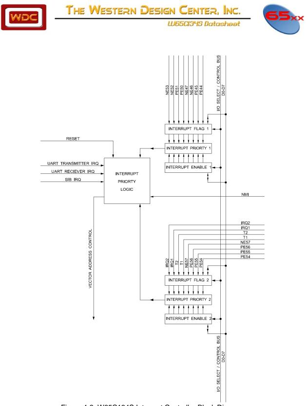
Figure 4-2 W65C134S Interrupt Controller Block Diagram
